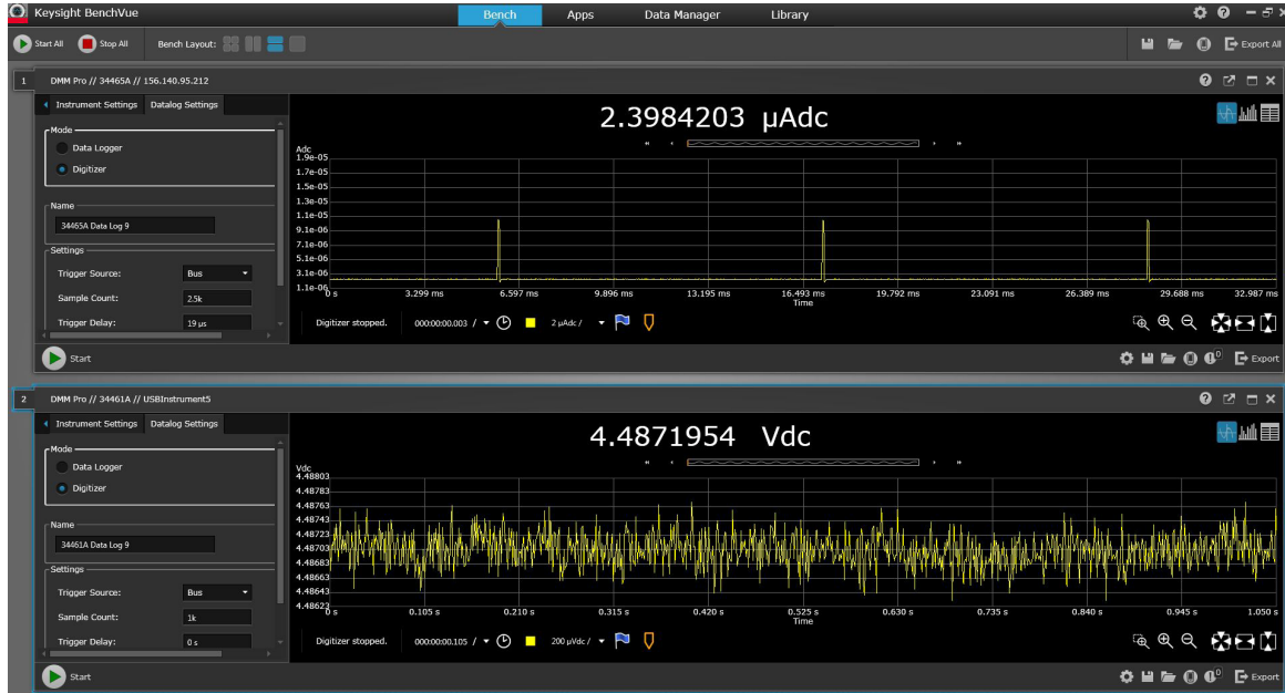
Figure 5. These two graphs illustrate the digitized DCI (top image) and DCV (bottom image) consumption
